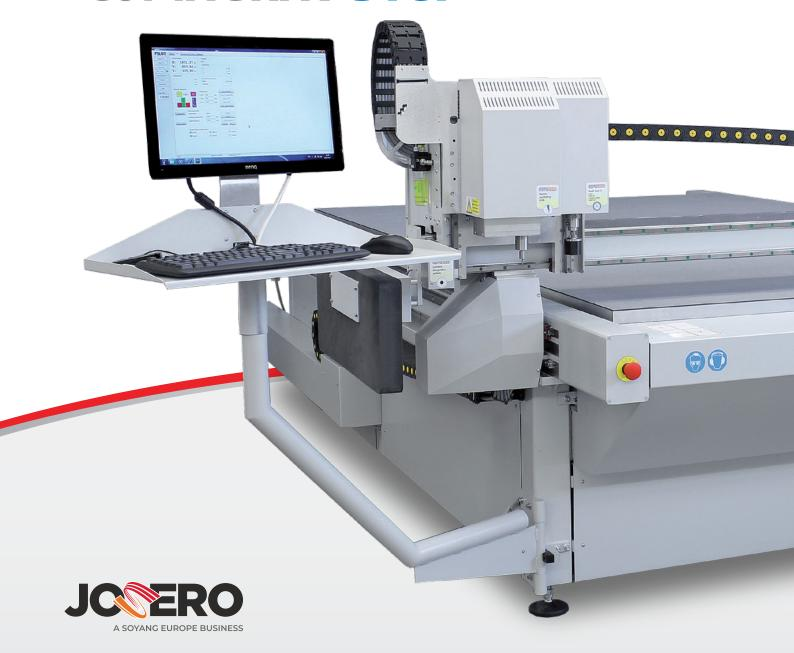
**COMAGRAV DIGI** is a powerful cutting table designed for cutting digital prints, corrugated cardboards, sandwich panels, sample making of packages, production of P.O.P. & P.O.S., cutting leather, nonwovens, PE foils, fabrics, banners, foams, etc. After successful years on market of CNC engraving and routing machines we developed machine that reaches the top level.
