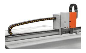
**COMAGRAV DIGI** camera system is standard on all models, it recognises printmarks and modifes the cutting path where necessary to allow for deformation or misplaced prints
