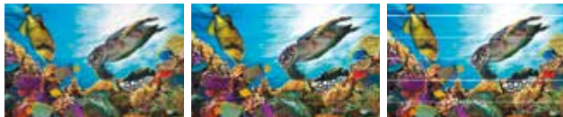
Incorrect bi-directional drop landing position
