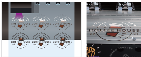
Designs are printed on a special adhesive film, and then an application sheet is automatically applied to the film.
