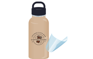
Peel off the application sheet. Once removed, the transfer is complete and the item is finished.
