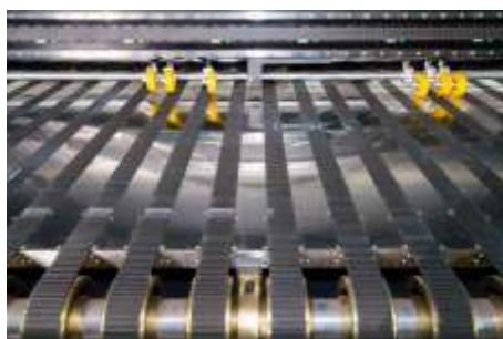
Stable Feeding: 22-zone full steel belt side suction platform automatic front-edge paper feeding mechanism.
